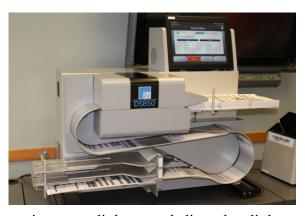
features of the DS850. While processing ballots, the DS850 prints a continuous audit log to a dedicated audit log printer. Reports are printed from a second connected printer. The DS850 saves voter selections and ballot images to an internal hard disk and exports results to a USB flash drive for processing with the Election Management System.
