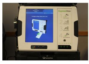
Each button on the tactile keypad has both Braille and printed text labels designed to indicate function and use to
