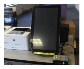
ICX DRE voting devices utilize the same user interface as the BMD counterpart. Instead of a ballot being printed on a standard piece of ballot stock, ballots are printed on a Voter Verified Paper Audit Trail (VVPAT) printer. The VVPAT serves as the official ballot for the voters using this device to cast their ballot and the ICX DRE is capable of tabulating ballots cast on the device.
