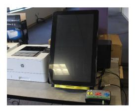
ICE X DRE voting devices utilize the same user interface as the BMD counterpart. Instead of a ballot being printed on a standard piece of ballot stock, ballots are printed on a Voter Verified Paper Audit Trail (VVPAT) printer. The VVPAT serves as the official ballot for the voters using this device to cast their ballot and the ICE X DRE is capable of tabulating ballots cast on the device.
