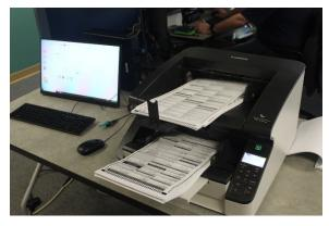
per minute. Reports can be printed from a separate connected printer. The ICC saves voter selections and ballot images to a USB flash drive for processing with the Election Management System.
