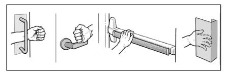
Door hardware can be used with a closed fist or open palm.
