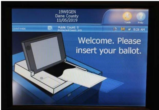
**Voter Information Screens:** The DS200 features a 12-inch touchscreen display to provide feedback to the voter regarding the disposition of any ballot inserted into the machine. The screens are designed to alert voters to errors on their ballot. The DS200 will, depending on the situation, provide details about the error, identify the specific contests where the errors occurred, allow the ballot to be returned to the voter, and provide the option for the voter to
