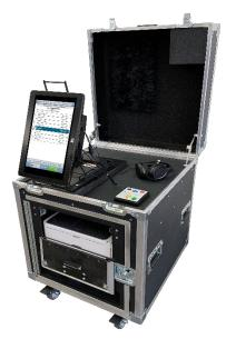
ClearAccess is an accessible touchscreen ballot marking device (BMD) primarily designed for use by voters who have visual, auditory, or physical limitations or disabilities. ClearAccess components include a touchscreen computer, a printer, and an uninterruptible power supply. All components may be implemented in a single wheeled case that can function both as storage and as a voting station at the polling place.
