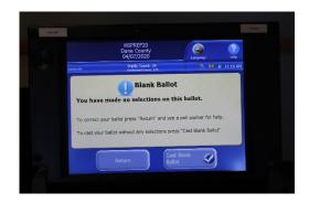
Error Scanning Ballot: If a ballot is inserted incorrectly, the DS200 will return the ballot to the voter and advise that the voter reinsert the ballot into the tabulator. The DS200 does not allow the voter to cast the ballot without resolving the issue and, if the issue persists, the voter is instructed to contact a poll worker for assistance.
