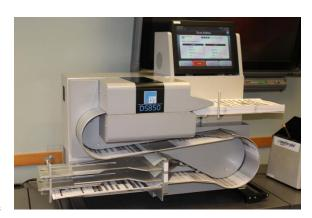
counted and may need to be remade by the election inspectors. Election officials use a 14-inch touchscreen display to program these features of the DS850. While processing ballots, the DS850 prints a continuous audit log to a dedicated audit log printer. Reports are printed from a second connected printer. The DS850 saves voter selections and ballot images to an internal hard disk and exports results to a USB flash drive for processing with the Election Management System.
