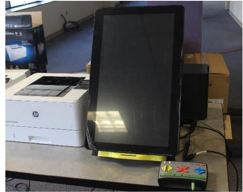
ICX DRE voting devices utilize the same user interface as the BMD counterpart. Instead of a ballot being printed on a standard piece of ballot stock, ballots are printed on a Voter Verified Paper Audit Trail (VVPAT) printer. The VVPAT serves as the official ballot for the voters using this device to cast their ballot and the ICX DRE is capable of tabulating ballots cast on the device.
