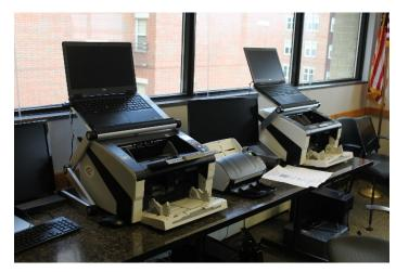
any other systems or the internet. ClearCount utilizes existing, off the shelf, Fujitsu scanner technology to capture an image of both sides of the ballot. All files that make up the ClearCount software reside on a single scan server that is shared by all the municipality's scan stations. The only software programs installed on the scan stations are the Windows operating system, the Fujitsu ScandAll Pro software and drivers required by the scanner hardware.
