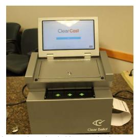
central office where the ballot images and election results may be uploaded into an election results management program or transferred to another memory device or machine to facilitate storage. ClearCast does not store any images or data in its internal memory.
