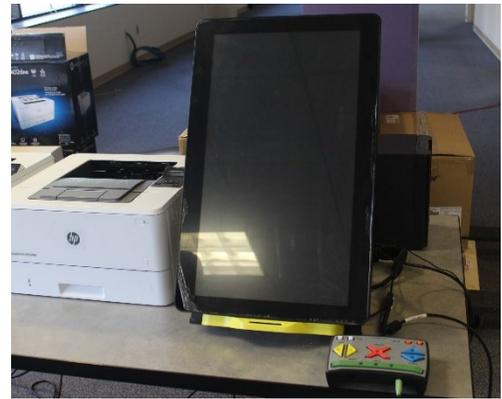
ICE X DRE voting devices utilize the same user interface as the BMD counterpart. Instead of a ballot being printed on a standard piece of ballot stock, ballots are printed on a Voter Verified Paper Audit Trail (VVPAT) printer. The VVPAT serves as the official ballot for the voters using this device to cast their ballot and the ICE X DRE is capable of tabulating ballots cast on the device.
